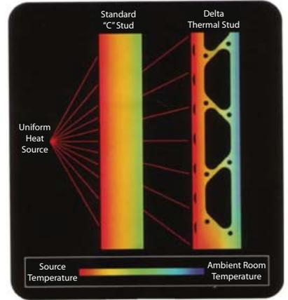
In a typical 8 foot section, Delta Stud shows 75% less thermal transference than "C" studs. Encased in structural foam, the thermal and structural performance of through-wall metal stud framing is unmatched.
