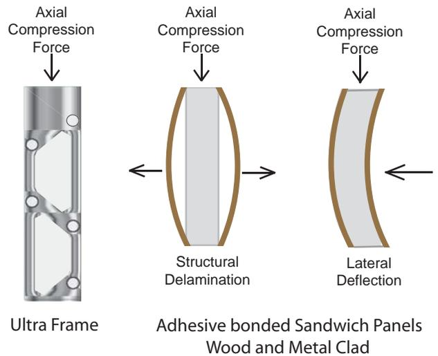
The result is an Ultra Frame building system that when exposed to fire, wind, and seismic forces will stand fast as most systems fail. The structural stud reinforcement of Ultra Frame increases the overall performance of the panel well beyond the competition.
